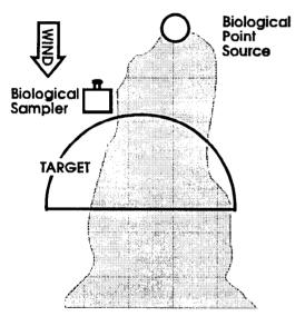
Figure 5-15b. Incorrect Placement of Sampler.
